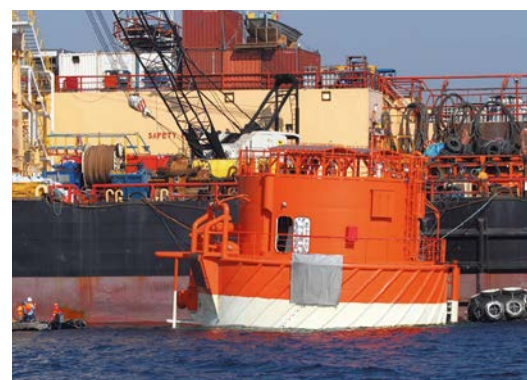
CPC is a pioneer in Russia in using the innovative method of tanker loading from single point moorings
